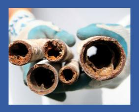
Piping is responsible for the delivery of compressed air to the point of use. Material, age and condition impact both system and air quality. Compressed air piping made from iron will rust and corrode, creating buildup on the interior and reducing the functional diameter. This buildup results in increasing pressure losses as well as contamination contributing to poor quality air.
